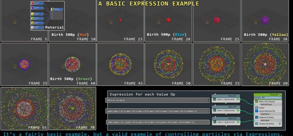
It's a fairly basic example, but a valid example of controlling particles via Expressions. The first thing we do, is birth bursts of particles every 10 frames using an 'if' statement. 2nd, we control the speed via a 'switch' statement ever the faster at later groups of frames. 3rd, we control the color of the particles via a 'switch' statement (6 different colors).
